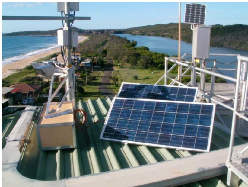
Figure1. The Wooli Beach Cams remote system incorporates 3 cameras and is solar-powered.
